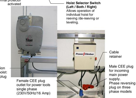
Connection plug to hoist: 10 pole plug
